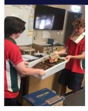
Miss Morgan's Year 10 Science class used a range of materials and techniques to design their own earthquake resistant buildings that would have minimal movement during an earthquake. Each group had the opportunity to test their buildings by shaking it in a box of mulch to simulate a real life situation. Afterwards the students evaluated the results.
